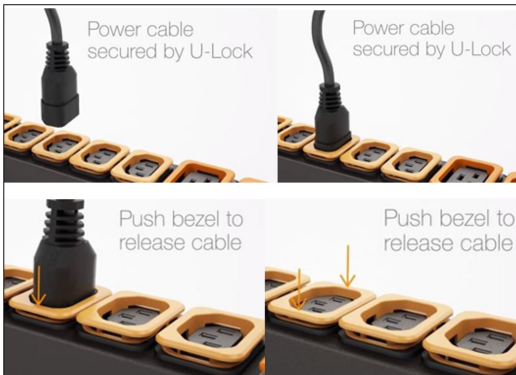
Figure 2.15 U-Lock Cord Retention Operation
