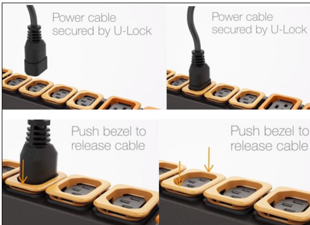
Figure 2.15 U-Lock Cord Retention Operation
