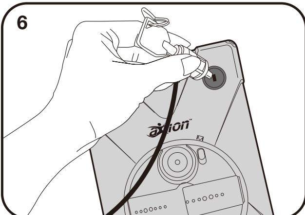
Insert the security cable into the security cable slot.
