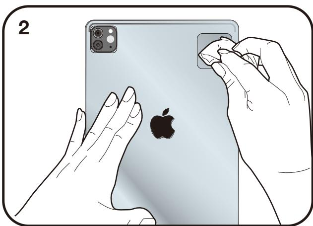
Using the included alcohol pad clean the surface of the device where the locking plate will install. The VHB adhesive adheres to the tablet properly when the surface is clean and dry.
