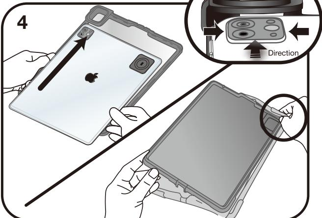
Install the tablet into the case by first installing the tablet into the plastic frame ensuring the raised camera is inserted UNDER the camera lens. Then, install the plastic frame and tablet into the silicone cover (reference the case installation guide for more detailed instructions).
