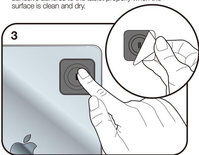
Apply the locking plate onto the tablet. Use an object to apply pressure and allow the adhesive to cure for 48 hours. Then remove the plastic template.
