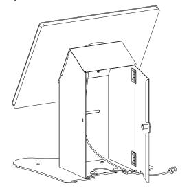
Unlock all back compartment using keys (C). Fish wire through the top to connect with device and out the bottom to your outlet or desired power source. Close door, insert key and rotate counterclockwise to lock.
