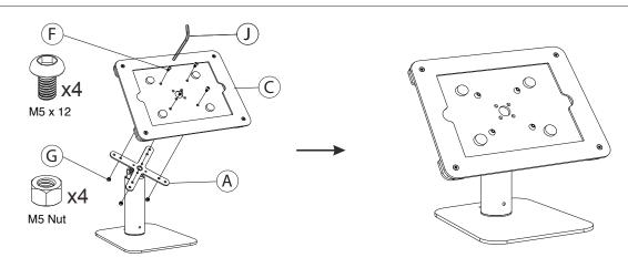
3A - Align enclosure VESA holes (C) to VESA plate holes of main body (A). Using provided tool (J), rotate in screws (F) from above while holding hex nut (G) from behind with your hands. Rotate until securely tightened.
