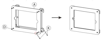
3E. Take the detached enclosure top (A), align the corner holes with the bottom portion. Then use (2) of the provided security star keys (K), turn in clock-wise the star screws (D) while holding the security star key (K) on the other side with your other hand. Screw in until securely tightened.
