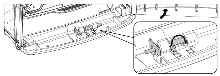
(6) Close and lock front door of Tech Tub<sup>2</sup> to secure devices
