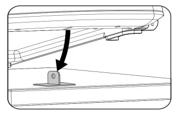
Open the front door and slide locking pin through metal tab
