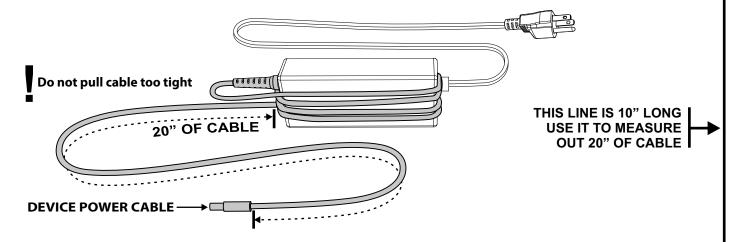
Wrap wall outlet power cable around power adapter leaving 6" of cable free
