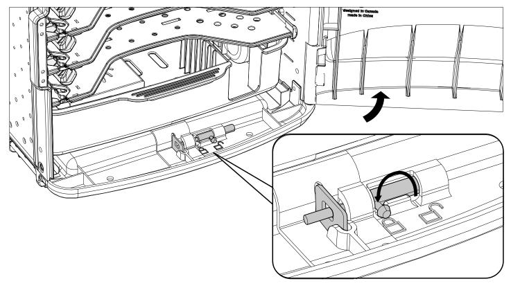
Close and lock front door of Tech Tub<sup>2</sup> to secure devices
