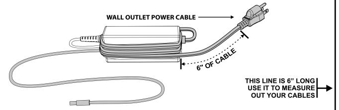
**③** Secure cables around adapter using provided hook and loop straps
