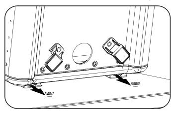
2 Fit slot (front underside of tub) over metal tab
