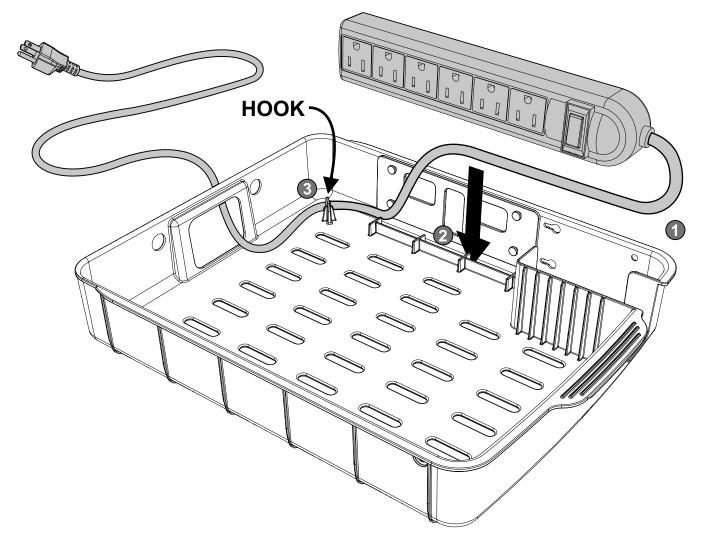
4 Fit 4 keyholes on Power Strip over 4 pegs on Power Strip Mounting Plate
