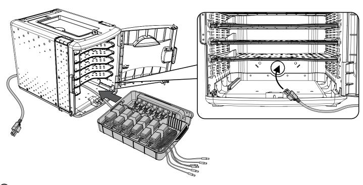
2 Partially slide Tray back into tub (leave a gap as shown below)
