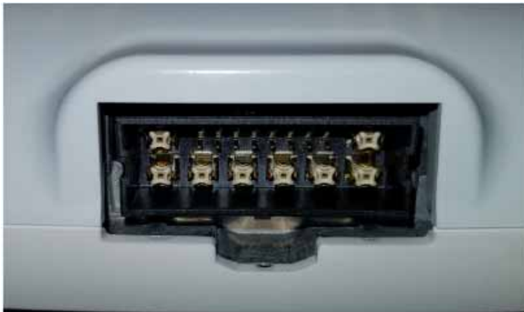
Figure 17 Smart Antenna Connector C9130AXE Model
