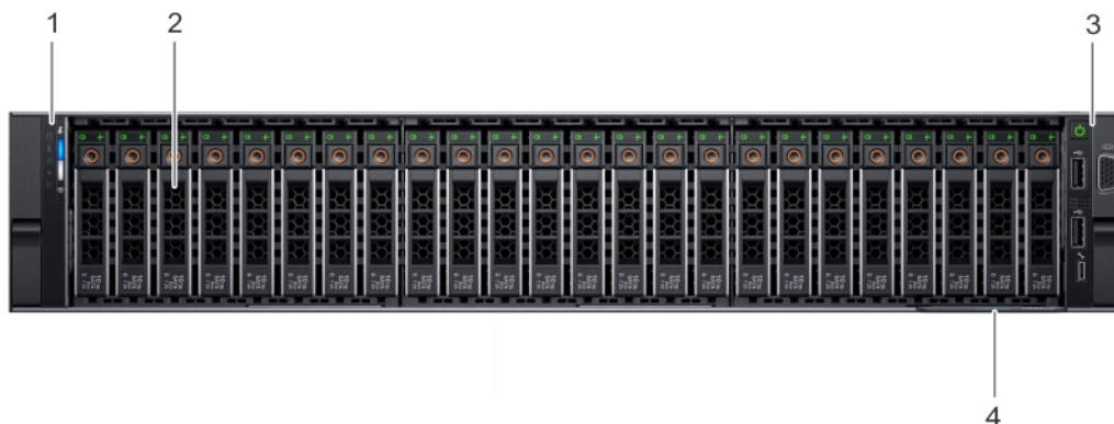
Figure 2. Front view of 24 x 2.5 inch drive system
