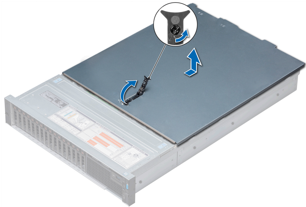
Figure 25. Removing the system cover
