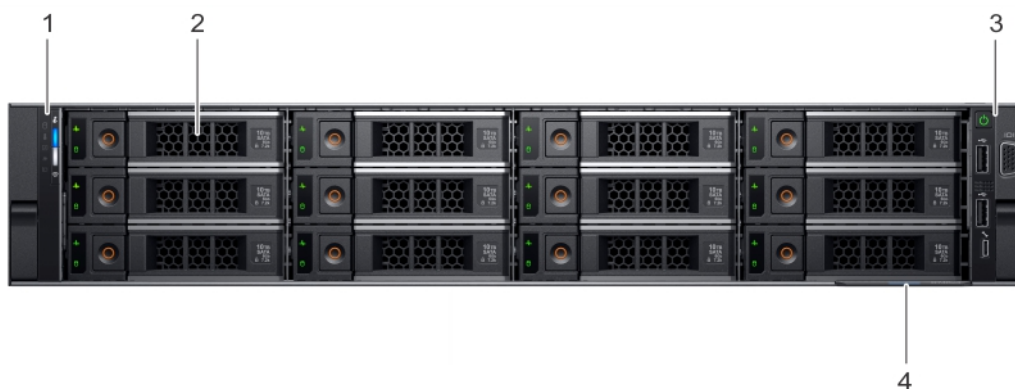
Figure 3. Front view of 12 x 3.5 inch drive system
