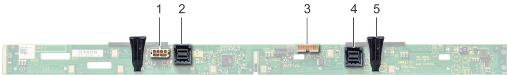
Figure 127. Back view of 3.5-inch backplane (mid drive tray)
