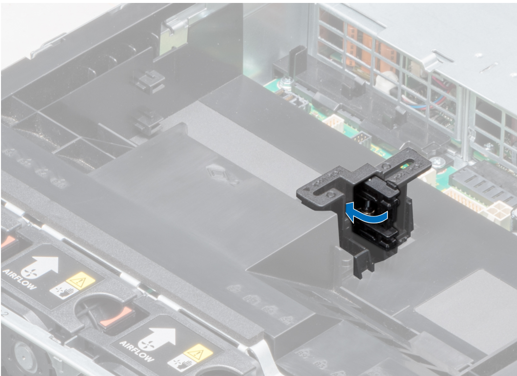
Figure 81. Closing the PCIe card holder latch
