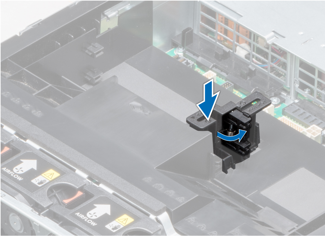
Figure 80. Opening the PCIe card holder latch
