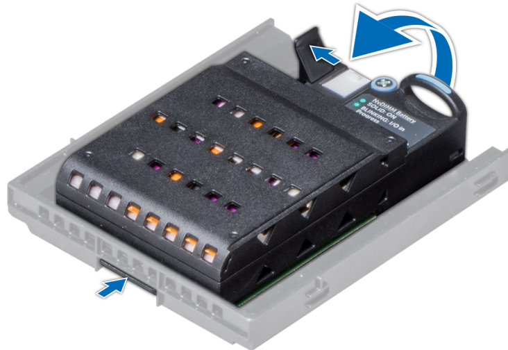
Figure 43. Removing NVDIMM-N battery from the bracket
