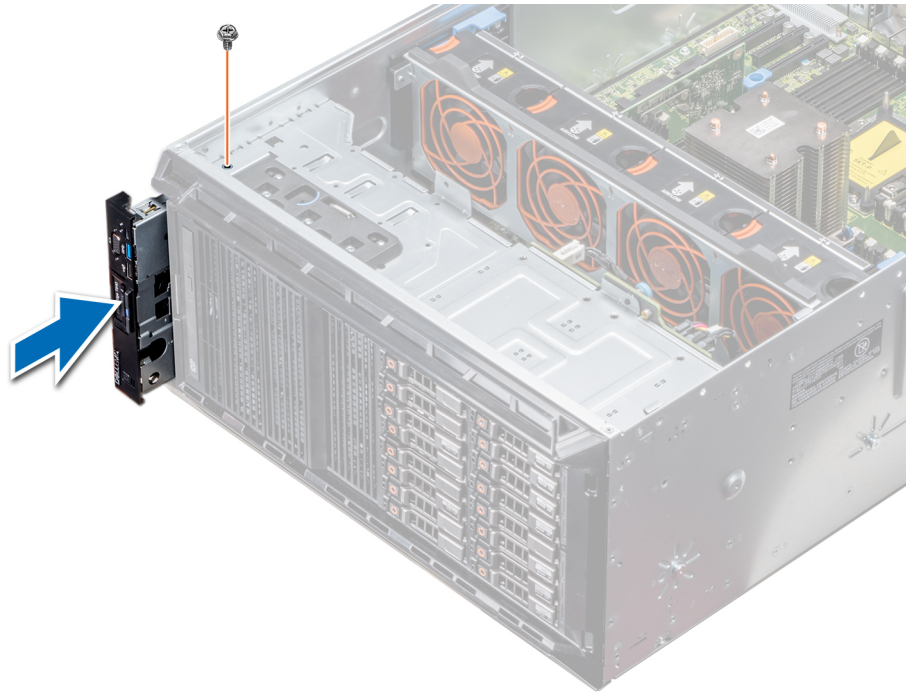
Figure 115. Installing the control panel assembly
