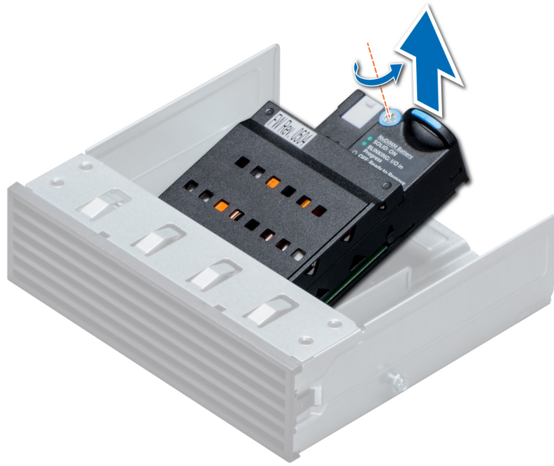
Figure 60. Removing the NVDIMM-N battery
