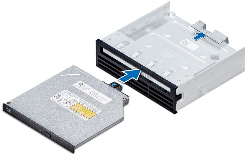
Figure 59. Installing the slim optical drive blank
