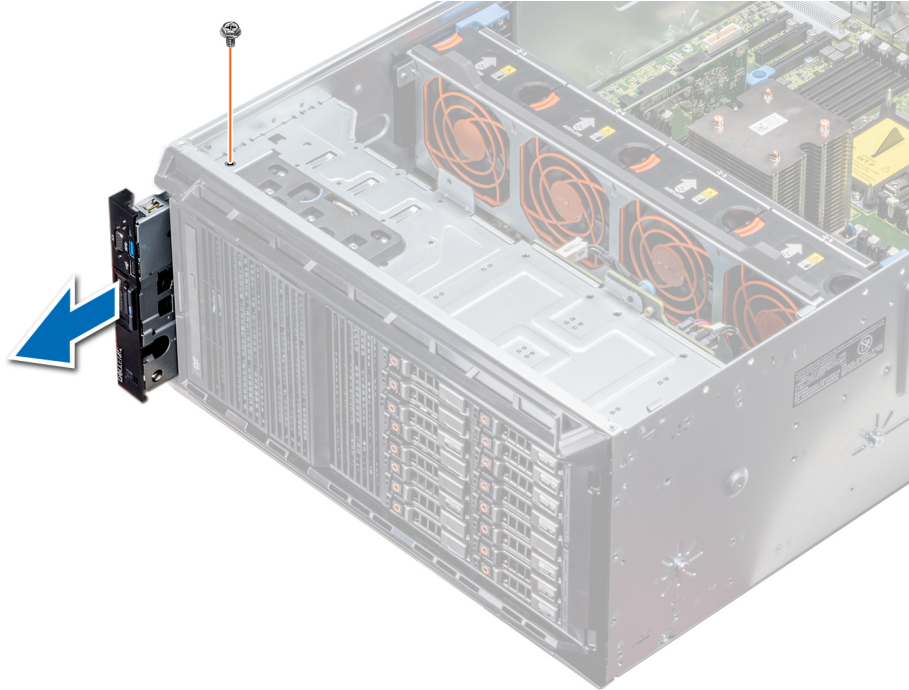
Figure 112. Removing the control panel assembly
