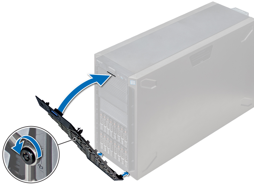
Figure 21. Installing the front bezel
