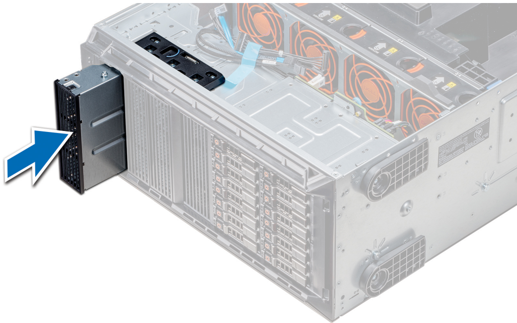
Figure 55. Installing the optical or tape drive blank
