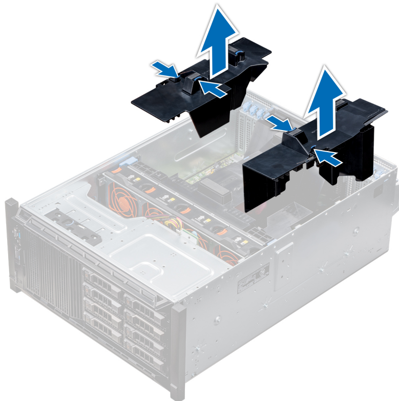
Figure 42. Removing the optional GPU air shrouds
