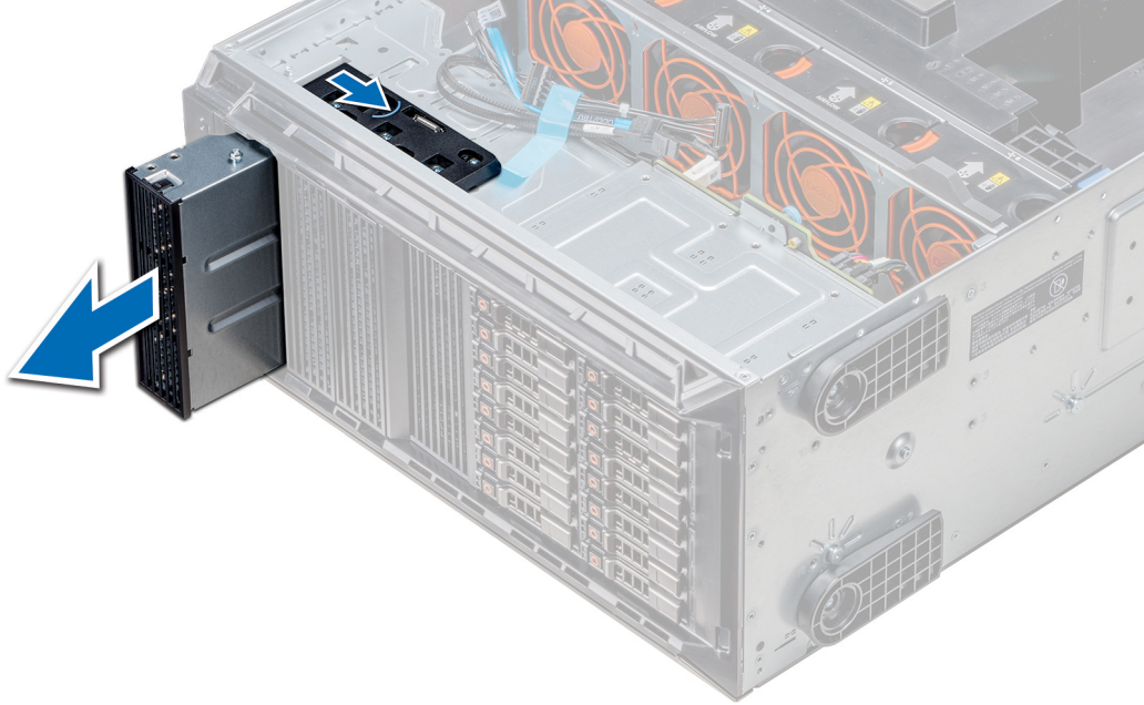
Figure 54. Removing the optical drive or tape drive
