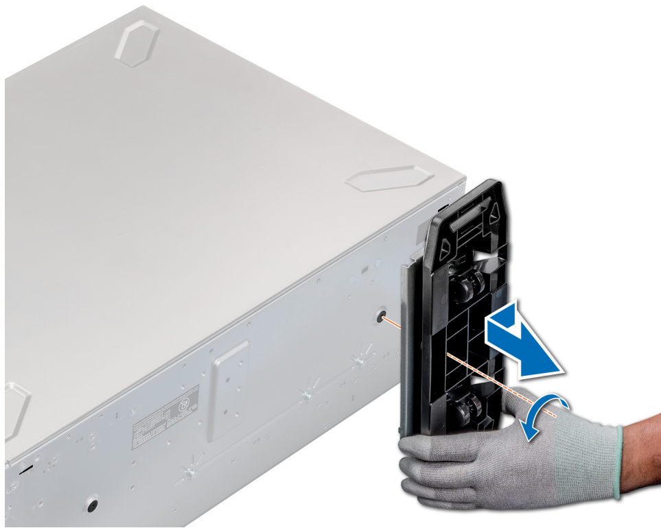
Figure 24. Removing caster wheels
