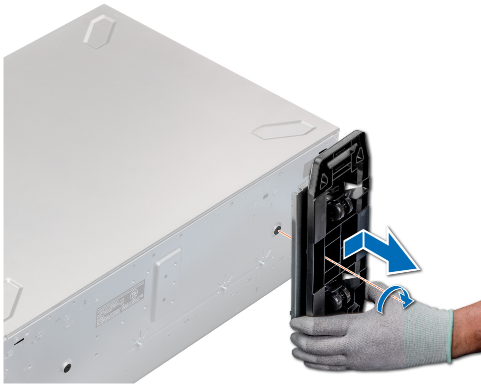
Figure 25. Installing caster wheels
