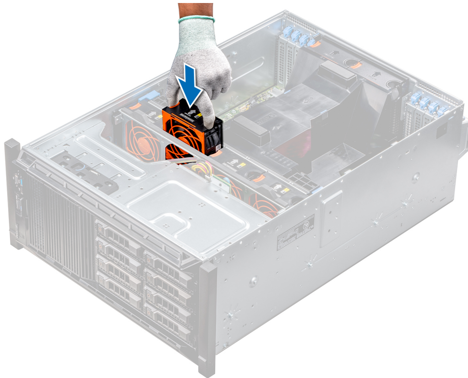
Figure 47. Installing a middle cooling fan
