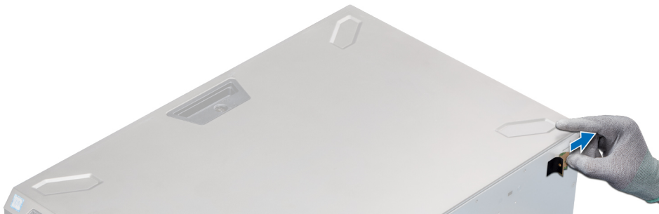
Figure 127. Attaching the mylar cover
