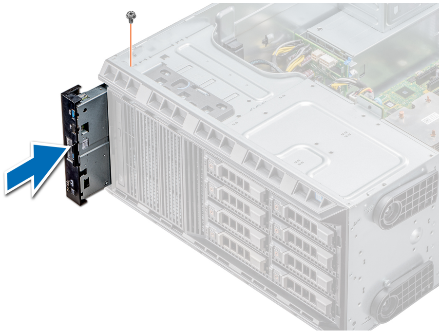
Figure 91. Installing the control panel assembly
