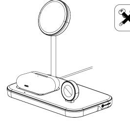
Mount your MagSafe Compatible iPhone device by placing it on the centre of the top charging pad ①. The integrated magnet will align itself to the phone once it has attached to the MagSafe Wireless Charging base.
