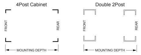
Step 2. 23.5" to 31.5": The Rear Rack Brackets will be installed as shown below for this "Mounting Depth" range (See Step 4 for assembly).
