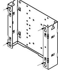
Step 3a. Install Drywall Anchor: Install one drywall anchor at each hole mark. Using a #2
