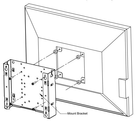
Step 9. <u>Attach Mount Bracket:</u> Attach the mount to the wall using the 4 screws that were installed in 3b. Secure by tightening screws.
