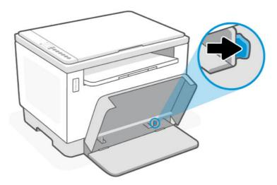
3. Insert the stack of paper into the input tray with the top forward and the side to be printed on facing up.
