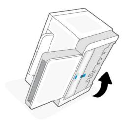
3. Release and hold on to the blue latch, and then remove the panel.
