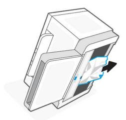
2. After clearing the paper jam, press the Resume button 1 to continue.
