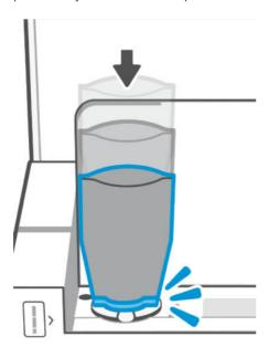
4. Rotate the refill lock ring counterclockwise until it stops.
