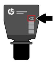
NOTE: You can identify the TRK with letter "X" (for High capacity) and letter "A" (for Standard) on the TRK.
