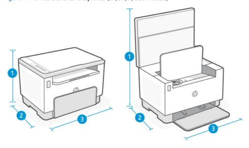
Table A-1 Dimensions for the printer (dn/dw/w/USB models)
