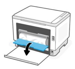
5. Hold the side edge of the paper and remove paper jam from the bottom first.
