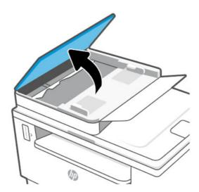
3. Remove any jammed paper visible in the input tray area. Use both hands to remove jammed paper to avoid tearing the paper.
