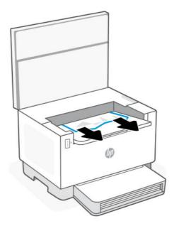
2. After clearing the paper jam, press the Resume button ( \sqrt{p}
