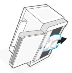
5. Hold onto the blue latch, align, and insert the panel. Release the blue latch to lock the panel in the place.
