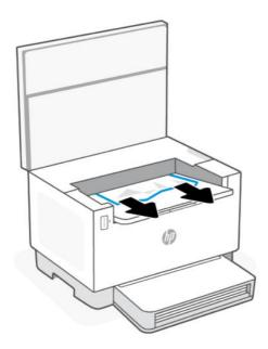
▲ CAUTION: Do not use sharp objects, such as tweezers or needle-nose pliers, to remove jams. Damage caused by sharp objects is not covered by the warranty.
