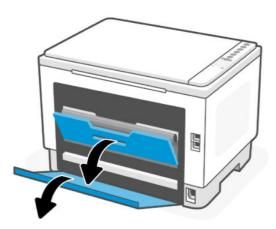
3. Open the scanner door, remove any visible jammed paper from the output tray area. Hold both the ends of the paper, pull gently towards you to avoid tearing the paper.
