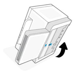
5. Release and hold on to the blue latch, and then remove the panel.
