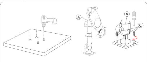
1A. Drill holes on the surface as shown above with power drill tool (not provided).
