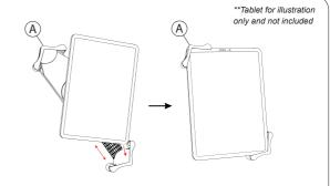
3A. Press quick release button on side of tablet holder (A) to release the adjustable end.
