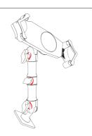
2. Adjust the arm to desired position then twist the screw knob clock-wise until securely tightened.
