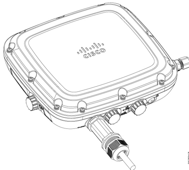
Figure 53: Fiber-Optic cable and gland installed to AP
