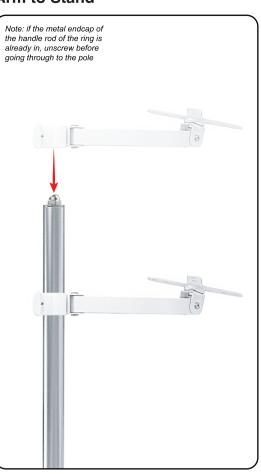
A. Loosen ADD-PARMVESA arm pole grip. Slide down to desired position then, tighten pole grip.
