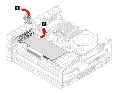
Note: Before installing a new PCI-Express card, remove any PCI-Express connector cables that impede the installation.
