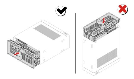
Note: Please push parts into the chassis completely until hear the sound of click.
