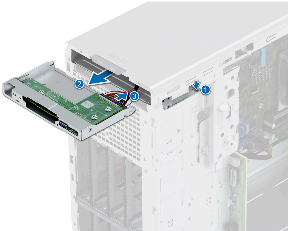
Figure 96. Removing the control panel cage
