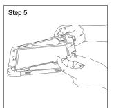
STEP 5: Re-insert the front frame back on. Make sure you go around the perimeter of the case and clip all the clips securely and tight.
