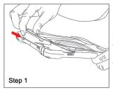
STEP 1: Peel away plastic frame starting with the bottom of the case as shown to the left. Work your way around the perimeter, unclipping the frame where there are clips.
