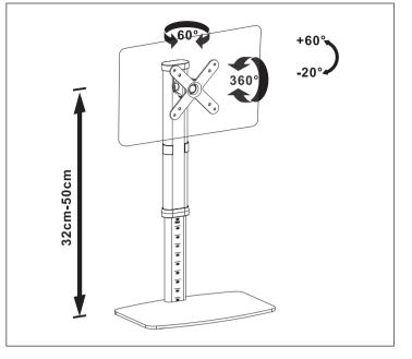
A. Using the included allen key tool, loosen the screw as illustraten above. Once screws are loosen, push up or down to adjust the height.
