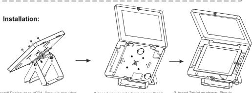
1. Install Enclosure to VESA. Screw in provided nails and nuts as illustrated (Shown Above)
