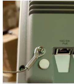
FIGURE 5 Attaching Security Cable to AP
