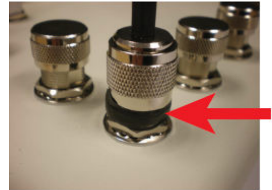
FIGURE 13 Wrapping the Exposed Connector Threads
