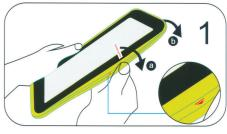
Remove the external silicone sleeve by peeling it away from the internal hard case
