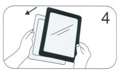
Once the iPad is inside the rear cover, place the internal front cover on top and gently clip all four sides into position.
