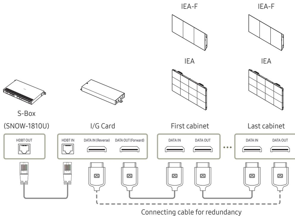
1 Connect the HDBT ports on the S-Box and I/G cards using a LAN cable.
