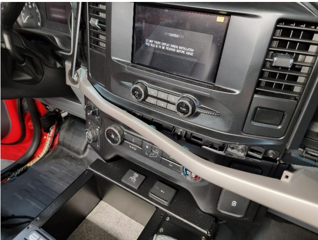
Temporarily reinstall the trim.
