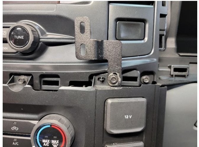
Install lower mounting tab using 7mm fastener.
