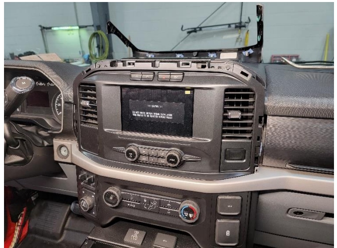
Remove trim around radio frame.
