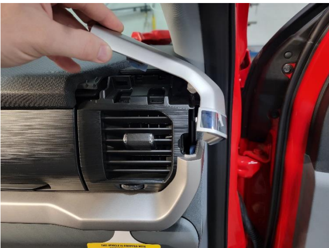
Unsnap trim around passenger vent assembly.
