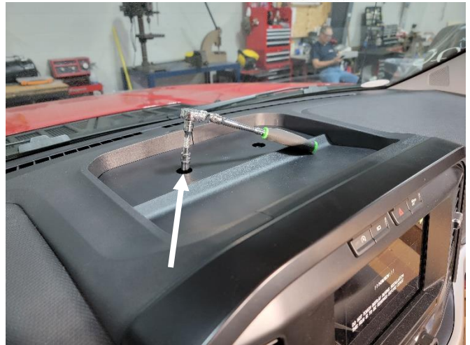
Remove (2) 7mm head fasteners at top center dash.
