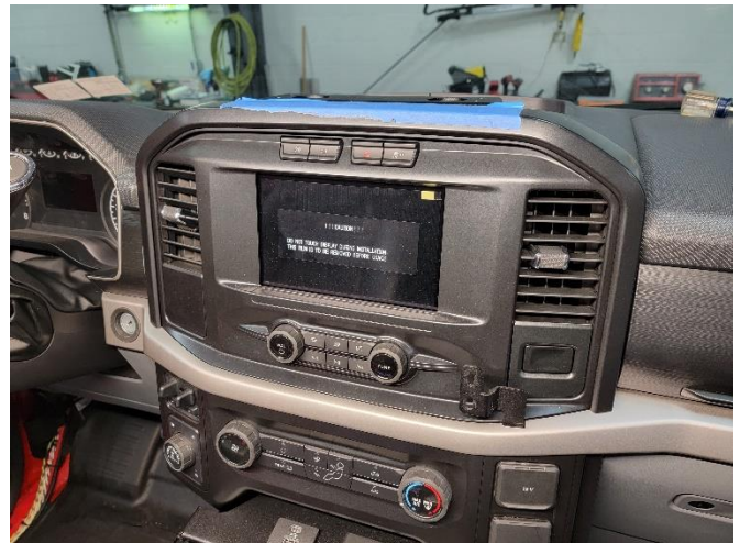
Reinstall previously removed trim around radio.
