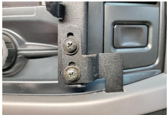
Attach frame support arm to lower mounting tab using (2) 10-32 x 1/2" machine screws, keps nuts and flat washers
