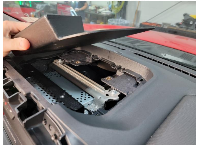
Place upper mounting tray onto dash.
