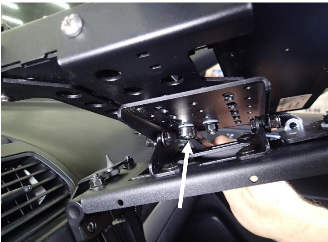
Determine desired position for your specific computer and attach to DMM swivel plate using 1/4"x 3/4" carriage bolts, PVC spacer, nylon washers, steel washers, and nylock nuts.
