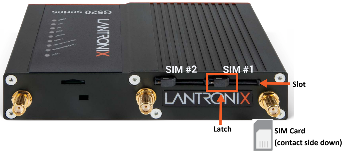
Figure 3-1 Inserting the SIM Card in slot #1
