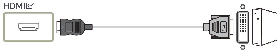
When using HDMI-DVI cable, audio may not be supported according to source device.
