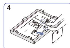
Push the assembled stand into the main body in the direction of the arrow as shown in the figure.
