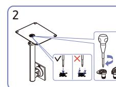
Put the stand base onto the stand neck as the direction shown in the figure. Check that the stand neck is firmly connected to avoid injury caused by falling of the base.
