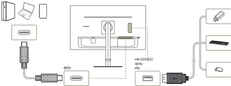
Using the product as a hub, connect and use various source devices with the product at a time.
