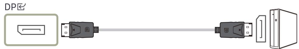
It is recommended to use the DP cable provided as an accessory. If not provided, be sure to use a DP cable of 1.5 m or below.
