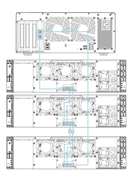
**2.** Connect the expansion units to the device using the following topology.
