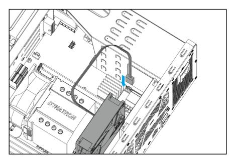
**c.** Attach the screws that secure the fan module to the chassis.
