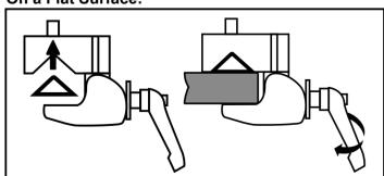
Place rubber grip flat insert into the clamp groove. Rotate tightening handle counter-clockwise to widen around surface ledge.
