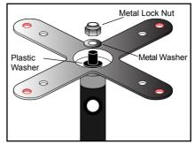
Place a plastic washer then a metal washer over the Pole tip, screw nut over to lock in place.
