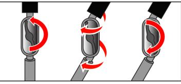
1. Loosen the Handle Rod of the Pole, Adjust the Pole to desired position then tighten the Handle Rod.
