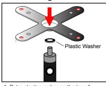
Put a plastic washer on the top of the Pole and then insert it into the VESA Plate.
