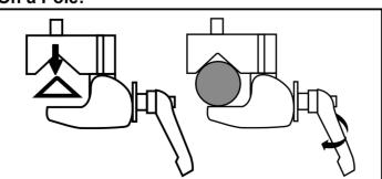
2. Remove rubber grip flat insert from clamp groove. Rotate tightening handle counter-clockwise to widen around surface ledge. Rotate clockwise to tighten until secure.
