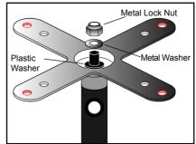
2. Place a plastic washer then a metal washer 3. Use the Socket Wrench to tigten it securely. over the Pole tip, screw nut over to lock
