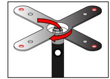
2. Rotate the VESA Plate to adjust it in horizontal.
