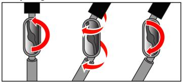
1. Loosen the Handle Rod of the Pole, Adjust the Pole to desired position then tighten the Handle Rod.
