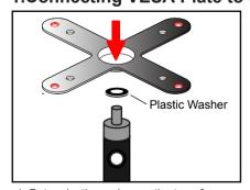
1. Put a plastic washer on the top of the Pole and then insert it into the VESA Plate.
