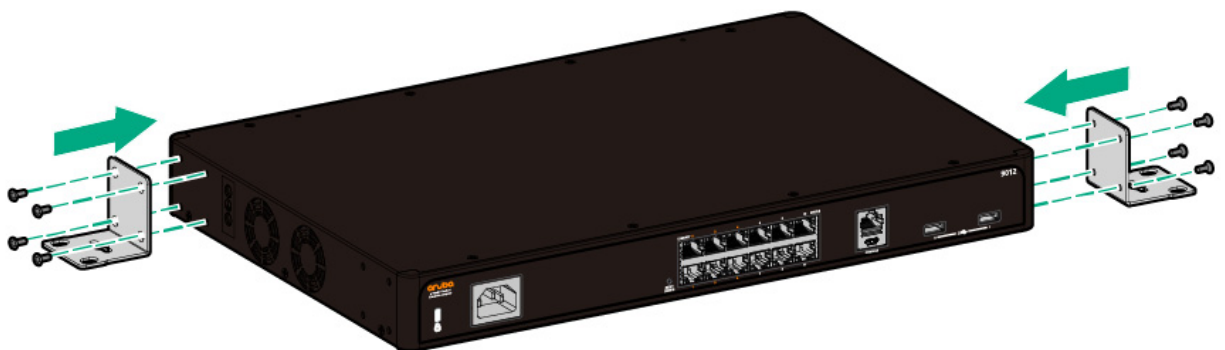
Figure 9 Attaching the Wall Mount Brackets
