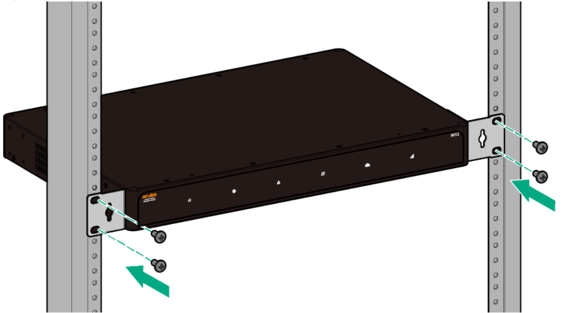
Figure 7 Rack Mount Installation
