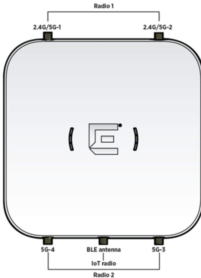
Figure 18: AP310e access point external antenna connector ports
