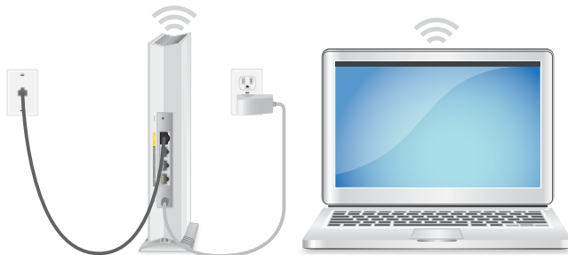
Figure 10. Connect the AP to an Ethernet wall outlet with Internet service
