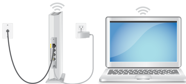
Figure 8. Connect the AP to an Ethernet wall outlet with Internet service
