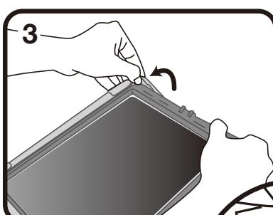
Insert the rest of the frame in to the cover.
