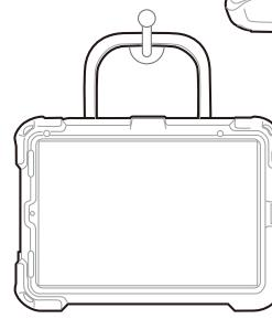
Insert each silicone tab tightly into its corresponding slot in the plastic frame to ensure the case is water-resistant.
