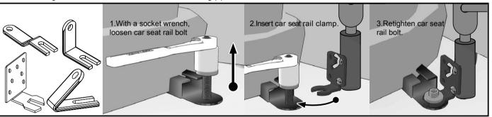
When connecting to the car floor or console - Use the (1) rail as shown below
