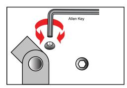
4B. When adjusting the hinge of the laptop holder use the tool provided as shown to loosen / tighten the joint as needed.
