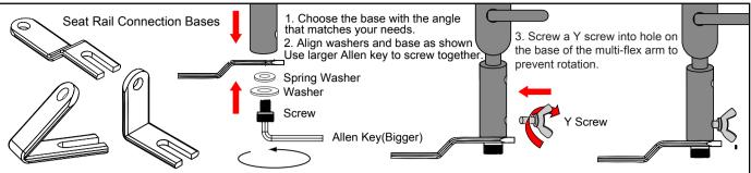
These two clamps allow you to connect the side of the Multi-flex pole
