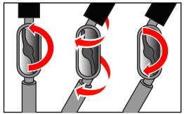
4A. Turn the knob counterclockwise to loosen any of the joints on the vehicle mount. Adjust the arm to the desired angle and position, then rotate clockwise to tighten and secure the position.
