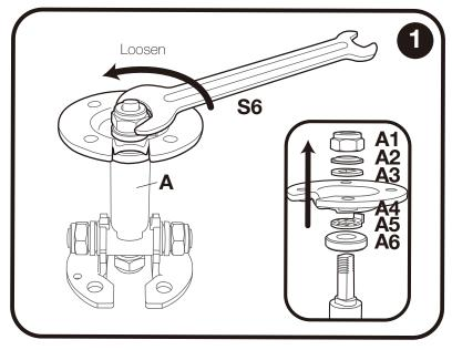
Using the included wrench(S6), loosen nut (A1) and remove all pieces (A1-A6).
