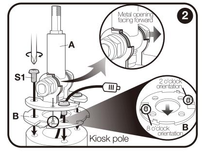
Place hinge (A) on top of plastic washer (B) & Kiosk pole. Install the 4 screws (S1) into the pole neck to secure the hinge down. Pull the cable out through the central hole of the kiosk and module.
