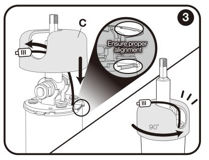
Install the hinge shroud (C) ensuring the bottom bumper meets the plastic washer gap (B), then turn the shroud 90 degrees counter-clockwise until it is locked.
