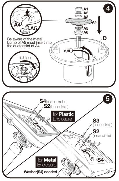
Slide the cover (D) onto the hinge, then reinstall and tighten all hardware (A1-A6) in the order shown.
