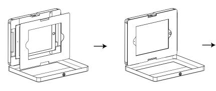
4. If needed, make sure to lay-in the correct masking cover. Then close and lock the enclosure and you're ready to go.
