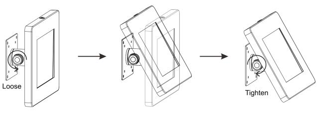
\*Rotate Counter Clockwise to loosen Ball Joint
