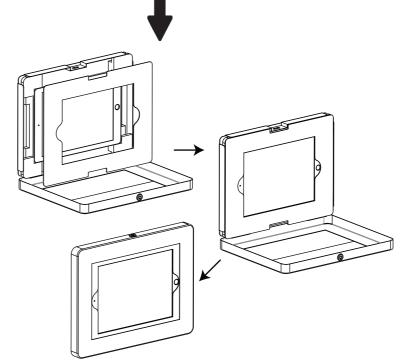
4 - If needed, make sure to lay-in the correct masking cover. Then close and lock the enclosure and you're ready to go.
