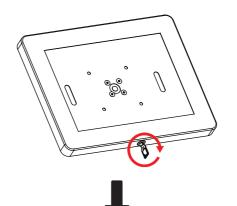
1 - Unlock the tablet enclosure by rotating the key until it pops open
