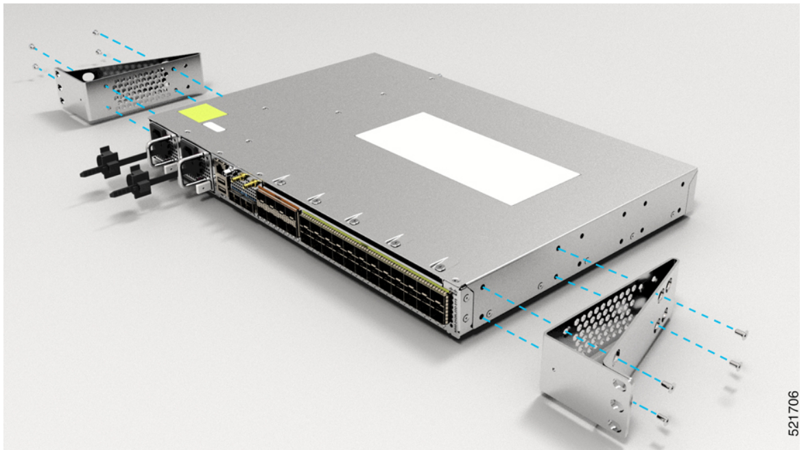
Figure 16: Installing ETSI Rack-Mount Brackets (N540-RKM-ETSI-FHC)
