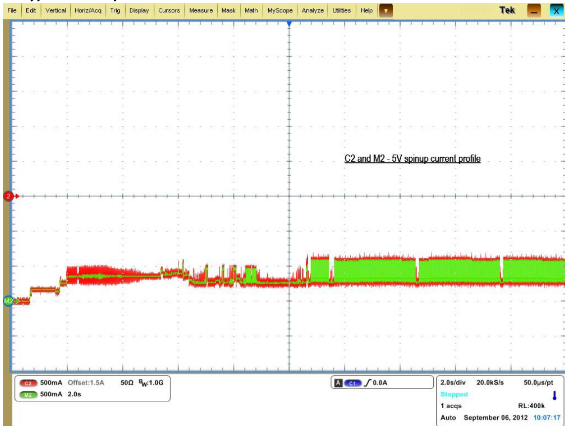
Figure 7. 1TB Typical 5V startup and operation current profile
