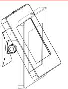
\*Adjust the VESA connection and the object fixed to the VESA to desired tilt and angle
