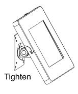
\*Rotate Clockwise to tighten and put the joint in a static state for use.
