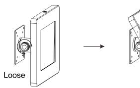
\*Rotate Counter Clockwise to loosen Ball Joint
