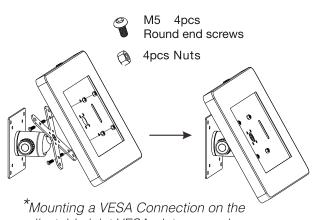
adjustable joint VESA plate example \*\*Tablet Enclosure is not included and only being shown as an example
