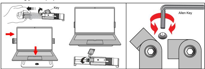
Insert key into lock at back of holder. Turn clockwise to unlock, then slide to open. Install Laptop against fixed end, then slide closed to hold tight. Turn counter-clockwise to lock, then slide to open. And you are ready to enjoy it.
