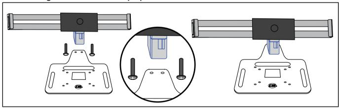
Screw up the screws by a screwdriver to connect the Holder to the Laptop Plate.
