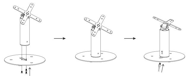
\*ALIGN HOLES AT THE BASE WITH THE HOLES ON THE BASE OF THE BODY. SCREW IN BOLTS WITH TOOL PROVIDED
