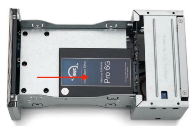
3. Affix the drive to the inner chassis. Holes for 3.5" drive screws are circled in red, and
