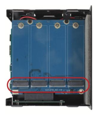
6. For each SSD you wish to install, remove the associated mounting screw from the circuit board. Then, align each M.2 SSD with its connector and slide the SSD forward until it is fully seated. If the drive feels stuck, do not force it into the connector; remove it, re-align the SSD's contacts with the connector and try again.
