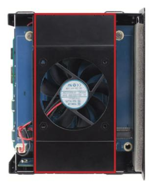
4. Remove the two fan housing screws (one on each side of the inner chassis), then disconnect the fan's power cable (outlined in yellow) from the circuit board. Set the screws aside then carefully lift the fan housing off the inner chassis and set it aside.
