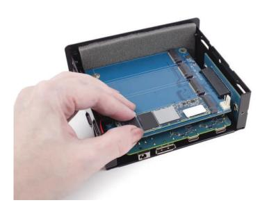
7. Each drive's mounting screw as shown. Repeat Steps 6 and 7 for each SSD being installed. The image below-left shows what the device looks like with all four M.2 SSDs installed. Note that you can use different brands and capacities of SSD if you wish.
