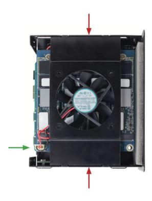
9. Align the inner-chassis with the track in the outer enclosure, then slide the inner chassis into the enclosure. If there is resistance do not force the inner chassis. Remove it, re-align it, then try again.
