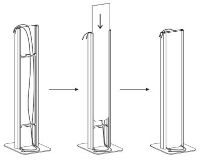
WITH ONLY (1) PANEL BACK IN, SLIDE IN THE POWER CORDS AND ANY OTHER CORDS THAT WOULD NEED TO BE CONNECTED TO THE TABLET THROUGH THE BODY AS SHOWN. THERE WILL BE GAPS AT THE TOP AND BOTTOM FOR THEM TO ROUTE OUT TO THE POWER SOURCE AND TO THE DEVICE. SLIDE IN SECOND PANEL WHEN ROUTING IS FINISHED.
