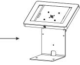
2. Screw in arm with tools provided for scanner holder component
