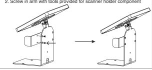
3. Use magnetic card reader holder component and place on metal surface as shown or anywhere
